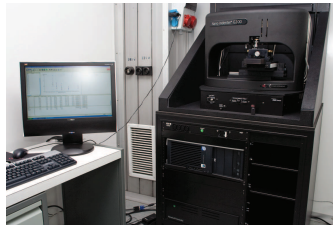
Nano Indenterul G200 (Agilent Technologies) aflat in functiune la IMT-Bucuresti
